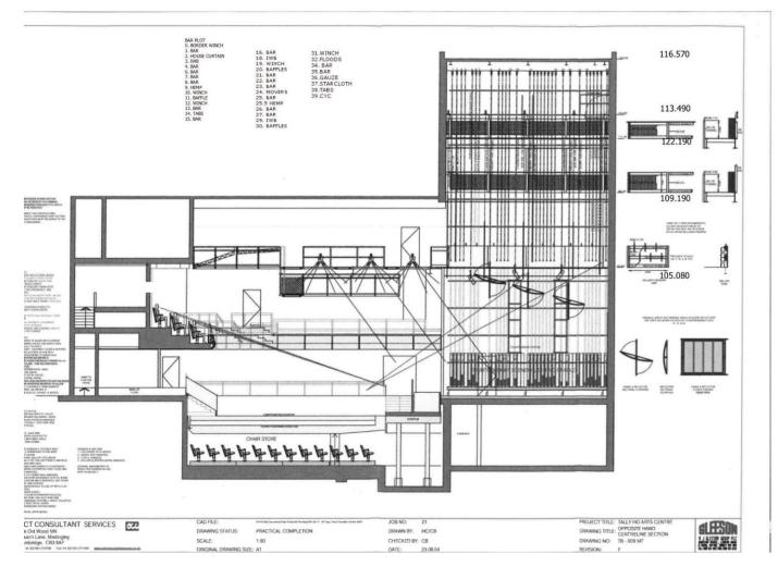
13.8m Proscenium fixed opening Proscenium adjustable opening 10.8m 2.4m left and right technical@artsdepot.co.uk // (020) 8369 - 5474 Wings Clear Stage Depth 9.15m Forestage depth 3.05m **Dimensions** Forestage width 10m Forestage (orchestra pit) 1.8m below stage Height of Proscenium 6.95m Stage height 0.88m Stage – underside of fly floor 6.85m Stage - grid 15.13m Auditorium – underside of FOH grid 7.82m Projection point – cyclorama 22.96m
